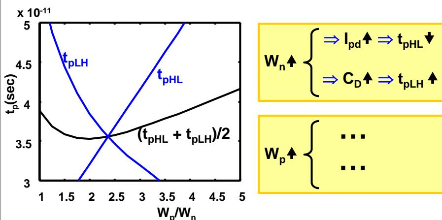
Min  $t_p$  in general not when  $t_{pLH} = t_{pHL}$
