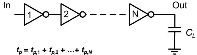
$$t_p = t_{p,1} + t_{p,2} + \dots + t_{p,N}$$
