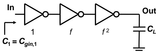
Delay per stage and total Path Delay
