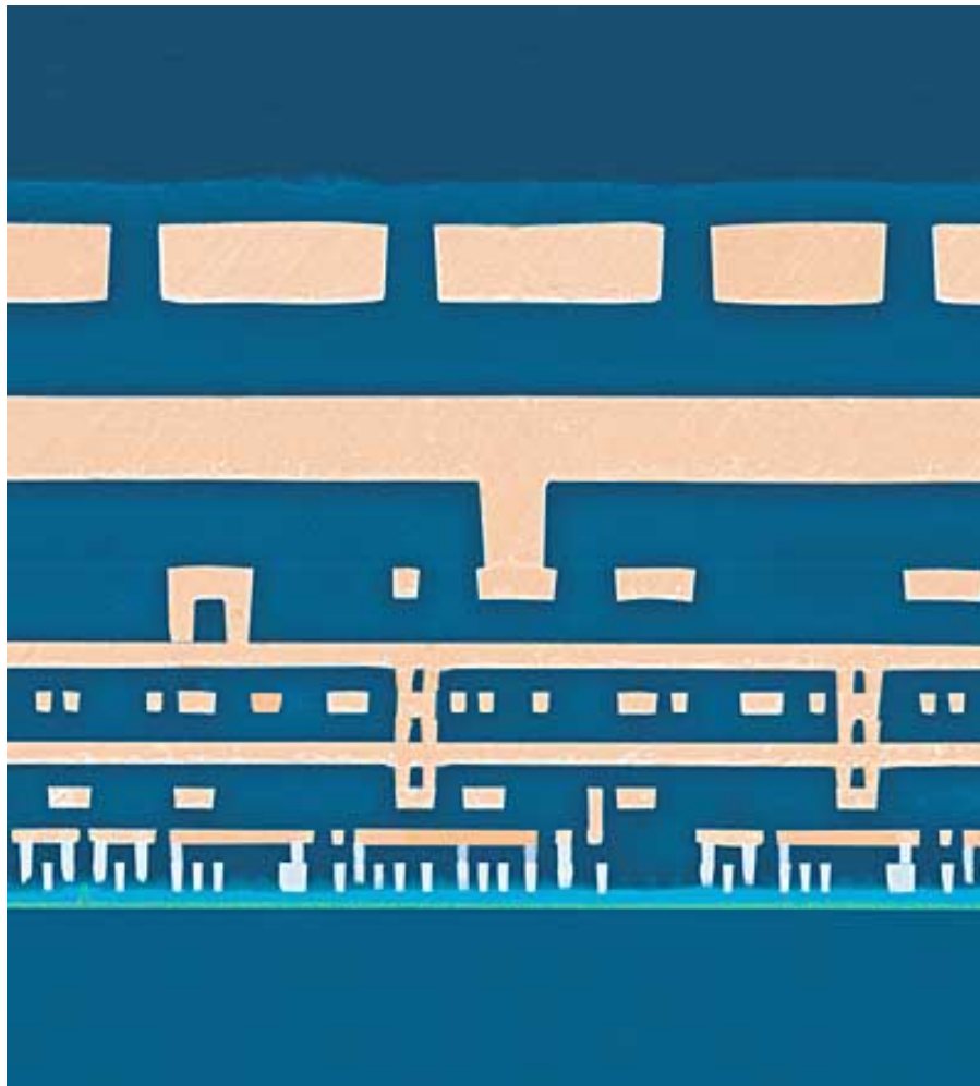
Cross-section of IBM 0.13 \mu process
