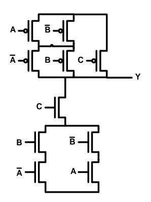
$$Y = \overline{\overline{A}BC + A\overline{B}C}$$
