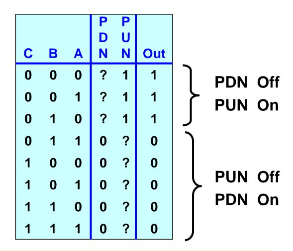
For all Complementary Static CMOS Gates, either the PUN or the PDN is conducting, but never both.
