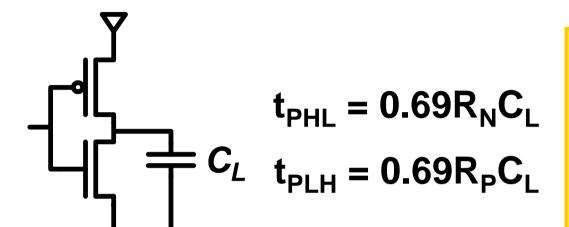
You should be able to identify the transistor paths that charge or discharge C<sub>1</sub>, and calculate resulting RC delay model, including effects of wires and fan-out
