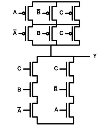
$$\overline{Y} = \overline{A}BC + A\overline{B}C$$
