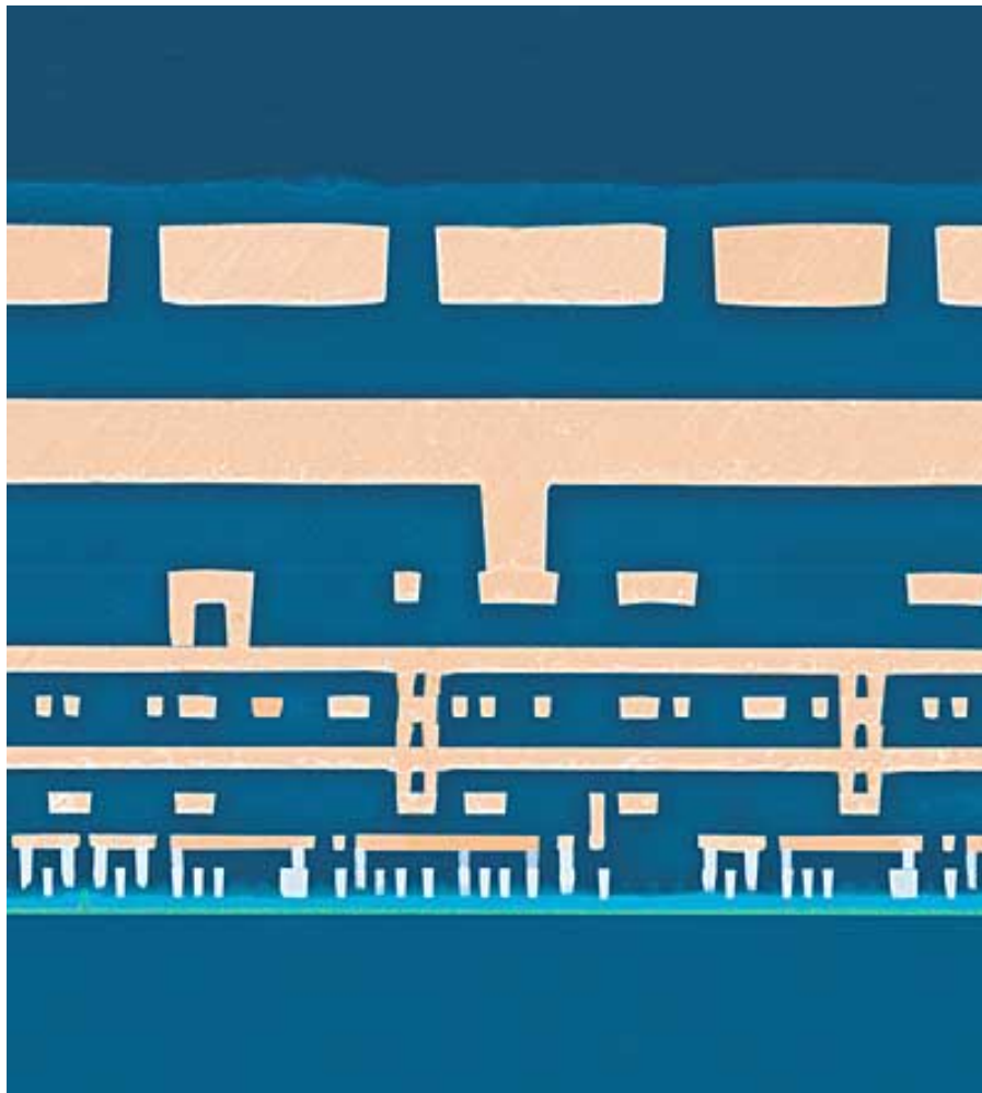
Cross-section of IBM 0.13 \mu process
