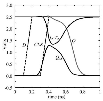
Slightly smaller delay between D and CLK
