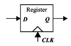
t<sub>c-q</sub>: delay from clock (edge) to Q
