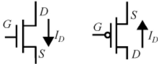
Figure 0.3 NMOS and PMOS devices.
