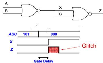
The result is correct, but extra power is dissipated
