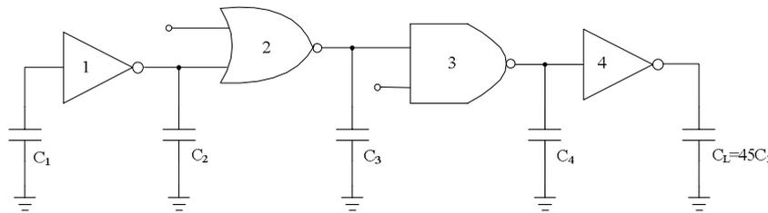
a. Calculate the optimum sizing for the logic circuit shown above.  $C_i$  denotes the gate capacitance of gate  $i$ . The size of gate  $i$  will be denoted as  $S_i$ . The load capacitance  $C_L$  is 45 times the gate capacitance of the first inverter  $C_1$ . Determine the sizes  $S_2$ - $S_4$  of gates 2-4 respectively (in multiples of the size of gate 1) that minimize the path delay. Assume  $\gamma = 1$ .
