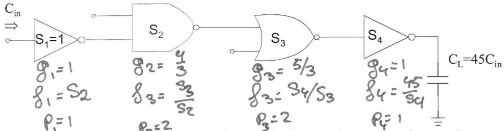
a. Calculate the optimum delay for the logic circuit shown above. Load capacitance  $C_L$  is 45 times the gate capacitance of the first inverter  $C_{in}$ . Determine the sizes  $S_2$ - $S_4$  and the minimum delay expressed in term of  $t_{p0}$  (intrinsic delay). Assume  $\gamma = 1$ .
