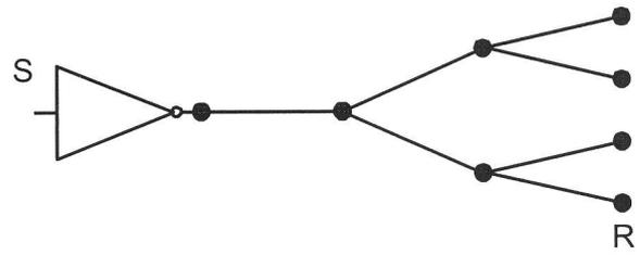
a. When the total capacitance of all segments together amounts to 1pF (which is not the correct answer to the next question), calculate the average current that the driver (the inverter) should deliver for a 50% delay of 1ns. For this question, please disregard the resistance of the wires. Assume  $V_{DD} = 2.5V$ .
