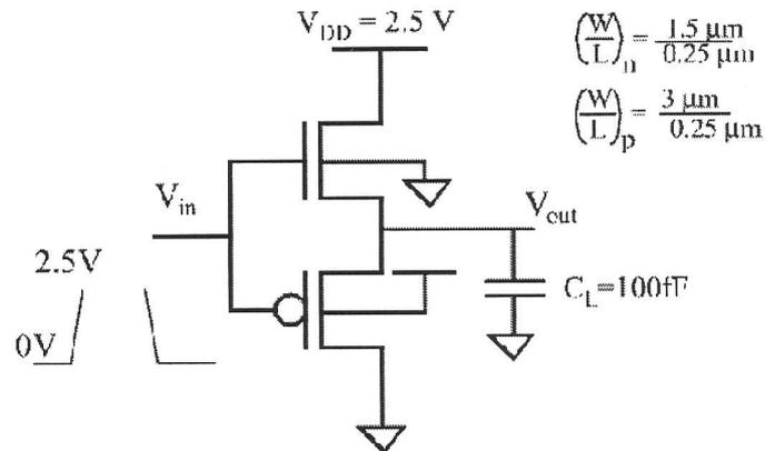
a. Write the equations for  $V_{OH}$  and  $V_{OL}$  taking into account the body effect in both transistors. First write it using symbols, than fill in numbers. You don't need to solve the equations.
