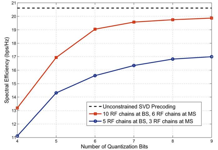
Fig. 10. Spectral efficiency as a function of phase quantization bits in a hybrid system with only quantized analog phase control. Results compare the performance of the hybrid analog digital channel estimation and precoding algorithms with the unconstrained digital system.
