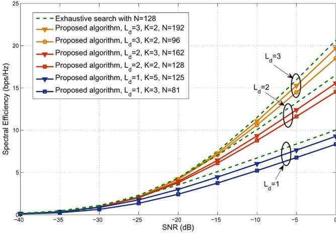
Fig. 7. Spectral efficiency achieved when the precoding matrices are built using the mmWave channel estimated by the proposed algorithms in a channel with  $L = 3$ , and  $L_d = 1, 2, 3$ . The figure compares the performance of the algorithm when different values of the parameter  $K$  are chosen. The results indicate that a very close performance to the exhaustive search case can be achieved with  $K \ll N$ , which maps to much smaller numbers of iterations.
