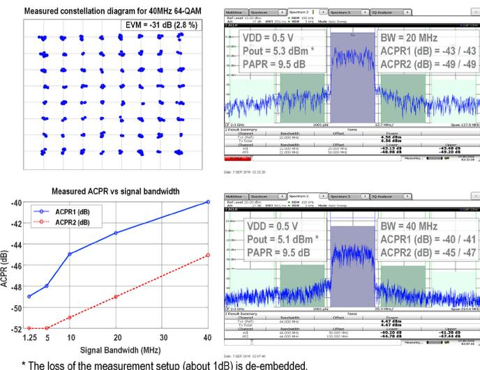
Figure 17.5.5: Measured 40MHz 64-QAM EVM and ACPR vs BW.
