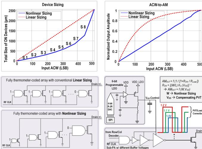
Figure 17.5.2: ACW-AM linearization concept and circuit.
