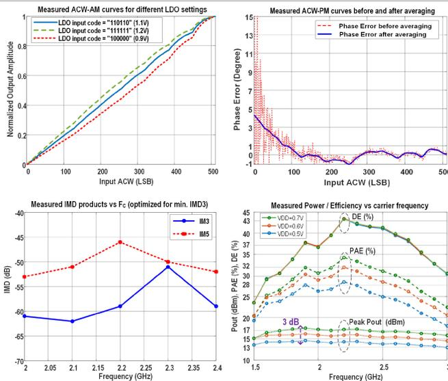
Figure 17.5.4: Measured ACW-AM/PM and Pout/DE/ IMD vs  $f_c$ .
