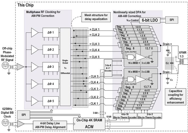
Figure 17.5.1: Overall block diagram of the linear DPA.
