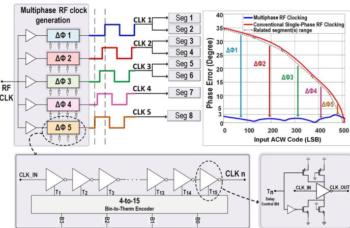
Figure 17.5.3: ACW-PM linearization concept and circuit.
