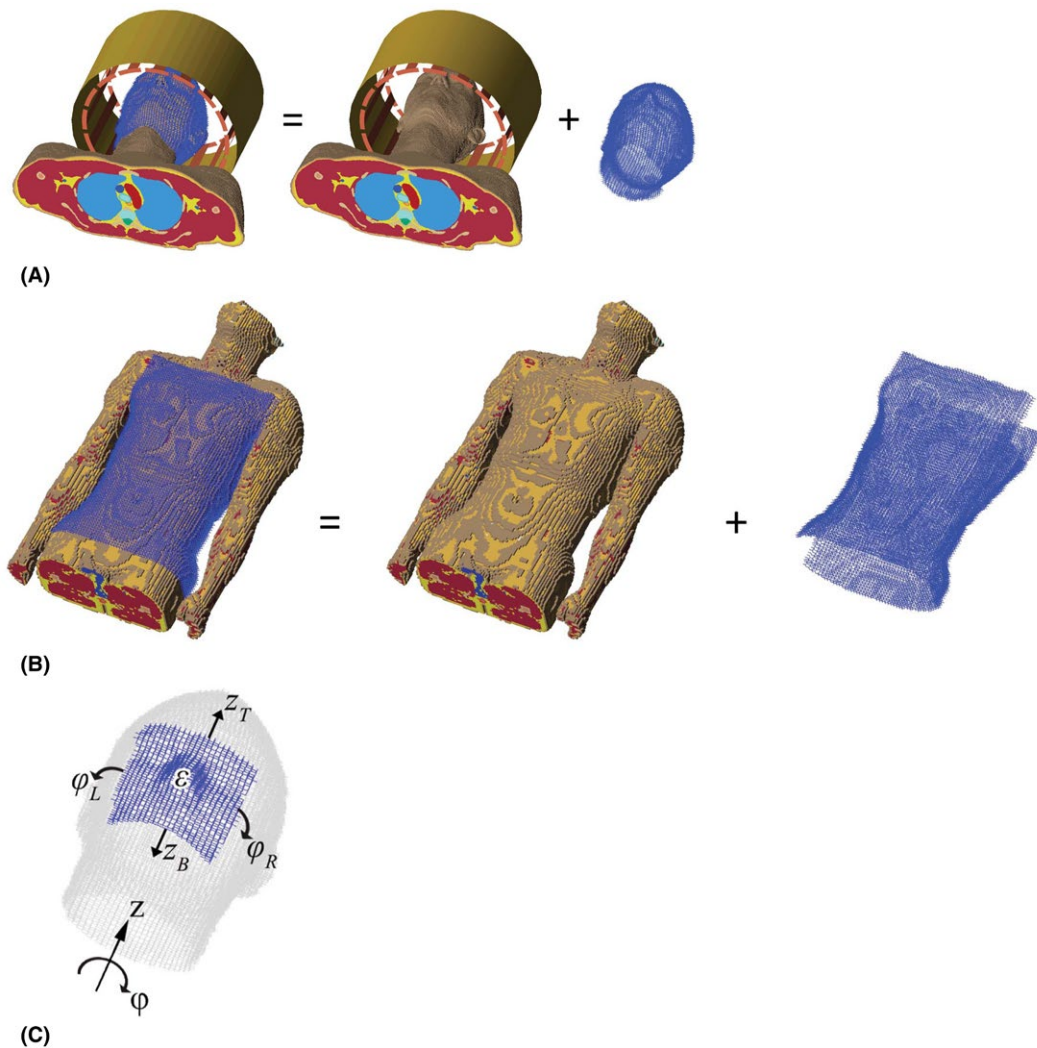
FIGURE 1 Splitting of computational domains and the parameterization of the dielectric pad. A, The 7T neuroimaging configuration is divided into a static part, consisting of a heterogeneous body model, RF coils, and an RF shield, and a dynamic part to which the dielectric is confined. B, The 3T body-imaging configuration is shown, here the wide-bore birdcage is omitted for visualization purposes of the pad design domain. C, As only the pads that can be easily fabricated are of interest, the model is parameterized in the pad's characteristics
