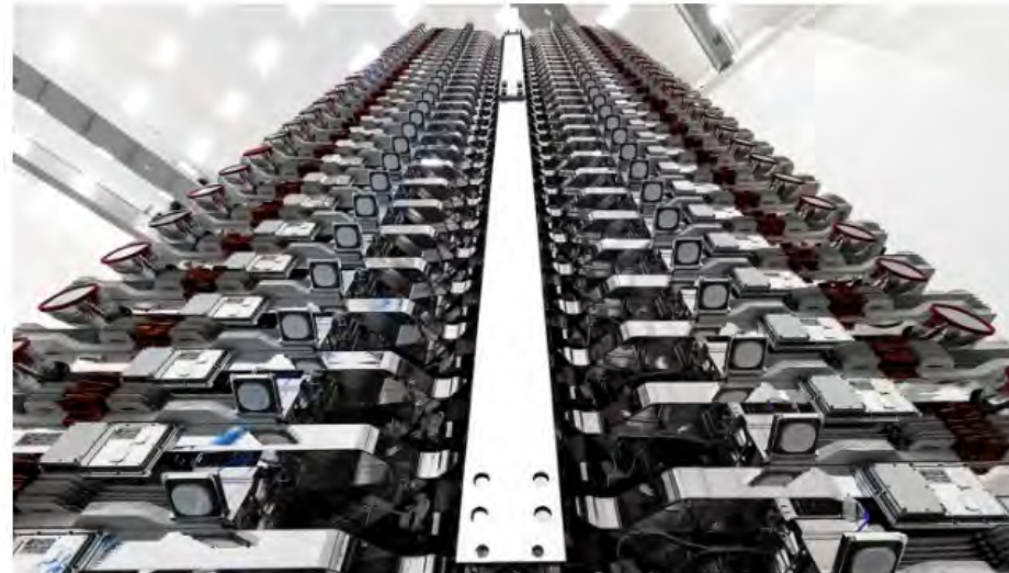
Sixty Starlink satellites packed into the nosecone of the Falcon 9 rocket SpaceX
