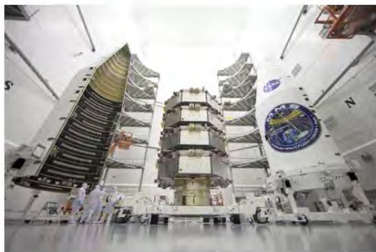
The four MMS satellites were stacked and packed inside an Atlas V rocket fairing in a clean room at the Astrotech Space Operations facility in Titusville, Florida. MMS is set to launch into space at 10:44 ET on Thursday night (March 12). Image released Feb. 19, 2015. (Image credit: NASA/Ben Smegelsky)
