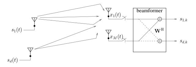
Assume we receive *d* signals on an antenna array, narrow-band case:
