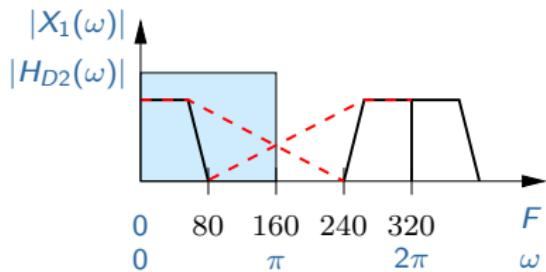
Here,  $\hat{N}_2 = 220$ , therefore, the total number of filter coefficients  $167 + 220 = 387$  is much smaller than the 5151 using the single stage implementation.
