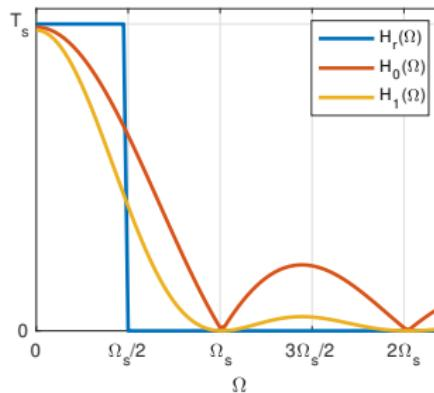
Due to the square, the linear interpolation filter will give much more suppression around  $\Omega_s$  and  $2\Omega_s$ .
