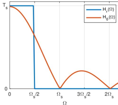
$H_0(\Omega)$  is not a sharp filter and aliased components around  $\Omega_s$ ,  $2\Omega_s$  will remain. The postfilter has to remove these.
