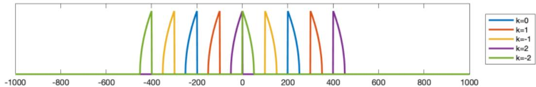
$m = 5$  is odd; the band  $F \in \{F_L \cdots F_H\}$  ends up at  $F \in \{0 \cdots B\}$
