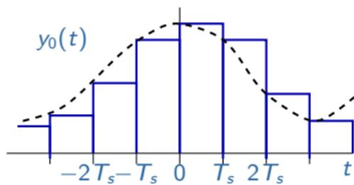
An analog postfilter (lowpass filter) smooths the step signal and removes remaining high frequencies
