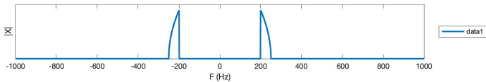
$$F_L = 200 \text{ Hz}, F_H = 250 \text{ Hz}, B = 50 \text{ Hz}, F_c = 225 \text{ Hz}$$
