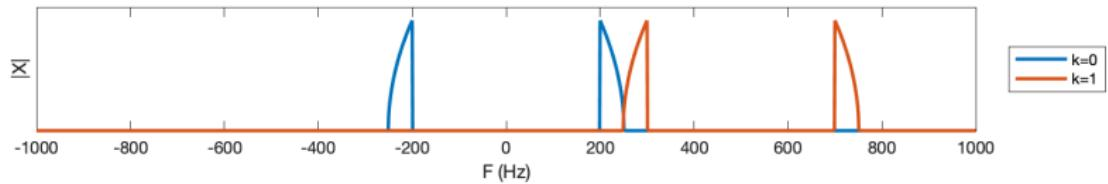
Most of the band is empty: not very efficient to sample at 500 Hz.
