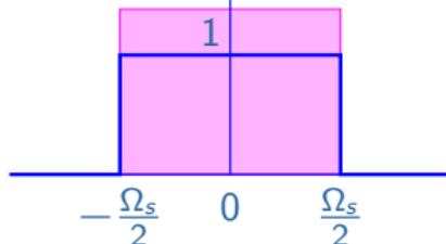
This prevents aliasing later during sampling. (The distortion of frequencies above  $\frac{1}{2}\Omega_s$  due to this filter is unavoidable.)
