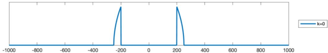
$m = 5$  is odd; the band  $F \in \{F_L \dots F_H\}$  ends up at  $F \in \{0 \dots B\}$
