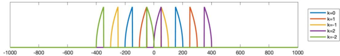
$m = 4$  is even; the band  $F \in \{F_L \cdots F_H\}$  ends up at  $F \in \{-B \cdots 0\}$ :
