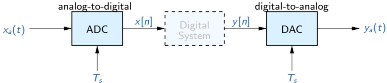
In absence of a digital system ( $y[n] = x[n]$ ), the goal for ideal sampling/reconstruction is to have  $y_a(t)$  equal to  $x_a(t)$ .
