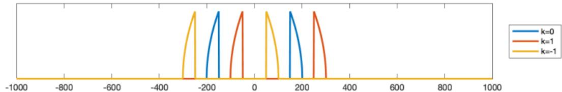
$m = 4$  is even; the band  $F \in \{F_L \dots F_H\}$  ends up at  $F \in \{-B \dots 0\}$ :
