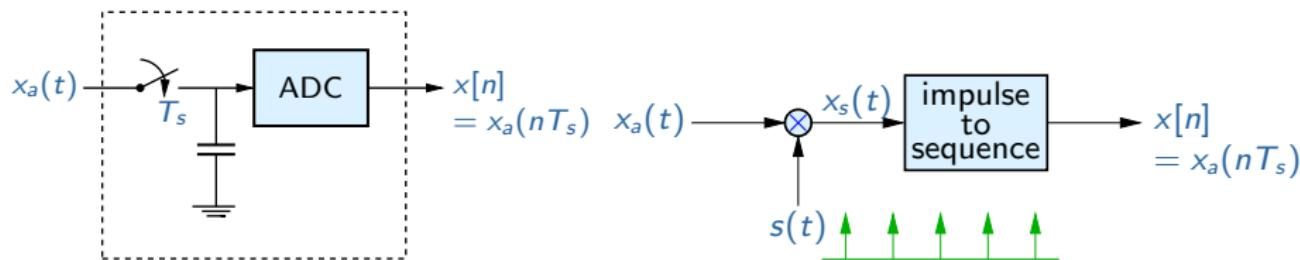
$T_s$  is the sampling period,  $F_s = \frac{1}{T_s}$  is the sampling frequency [Hz].
