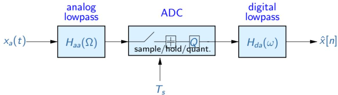
The hold circuit is often based on a capacitance (buffer) to maintain the voltage. The switch is often a MOSFET transistor.
