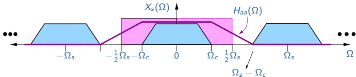
After sampling, we can digitally filter out the undesired components between  $\Omega_c$  and  $\frac{1}{2}\Omega_s$ .
