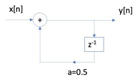
The quantization that takes place after multiplication uses N=3 bits and rounds up (i.e., if the value to be quantized is equal to the decision threshold, and therefore it is at equal distance from 2 quantization levels, the higher quantization level is assigned). Due to the quantization, the system does not produce the ideal output y[n]; instead, it produces v[n] as
