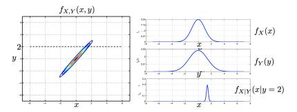
With observation y = 2, the posterior density  $f_{X|Y}(x|y)$  is very concentrated around  $\hat{x} = E[X|y = 2] \approx 1.5$
