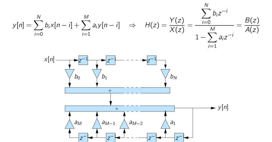
This is not a minimal structure  $(M + N \text{ delays instead of } \max(M, N) \text{ delays})$ .
