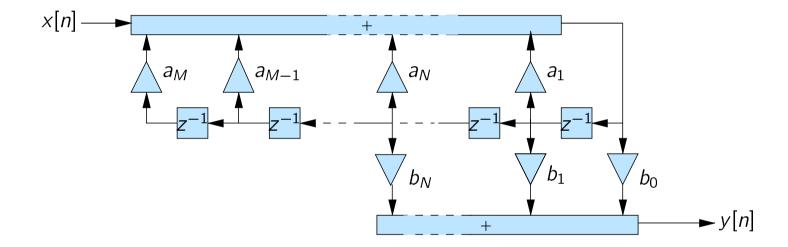
The filter coefficients are directly related to the parameters of the difference equation.
