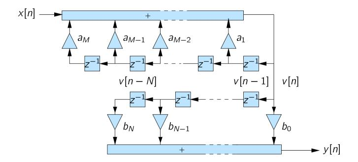
Notice that the delay lines can be merged (they transport the same signal v[n])
