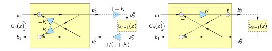
The number of multiplications can be further reduced by the following transform (the closed-loop response does not change)
