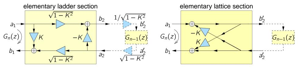
The elementary section is an orthogonal matrix (rotation):
