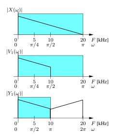
1.5p (c) Multiplication (modulation) with  $e^{j\omega_0 n} = (-1)^n$  in time domain corresponds to shifting by  $\omega_0 = \pi$  in frequency domain. Hence, the spectrum of the lowpass filter  $H(e^{j\omega})$  is shifted by  $\pi$  and it becomes a highpass filter.
