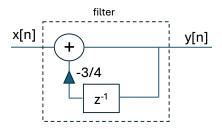
In the implementation of the filter, the output of the multiplier is quantized to 3 bits plus a sign bit using sign-magnitude representation. The range of the quantizer is [-1, 1]. The result is rounded downward in case it is equal to the decision threshold.
