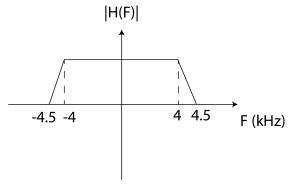
(2p) (f) (1 point) The useful part of the signal is between 3-4kHz. Aliasing must not affect this range, but may affect 4.5-6kHz.
