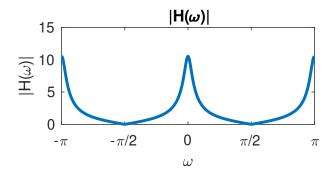
Peaks at  $\omega=0,\pi$ . The peaks have equal heights, due to symmetries. At the peaks the function is flat (hard to see in the matlab plot, but you can indicate this more clearly in the sketch). Evaluate  $|H(\omega=0)|=\frac{2}{0.1\cdot 1.9}=10.530$ .
