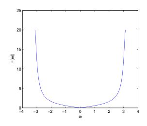
High-pass. Zero at z = 1 results in  $H(e^{j\omega}) = 0$  for  $\omega = 0$ . The pole at z = -0.9 results in a peak for  $\omega = \pm \pi$ . The pole at z = 0 only has an effect on the phase. Compute:  $H(e^{j\pi}) = H(1) = 20$ . (However, the pole-zero plot does not specify the gain so this value is actually unknown.) The shown plot should be symmetric and either plot from  $-\pi$  to  $\pi$ , or show periodicity outside this interval.
