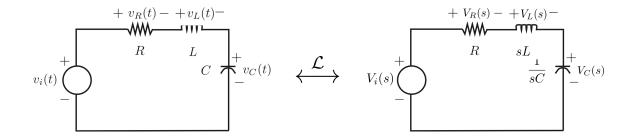
Let  $H_L(s)$  denote the transfer function of the (input) voltage source to the (output) voltage across the inductor,
