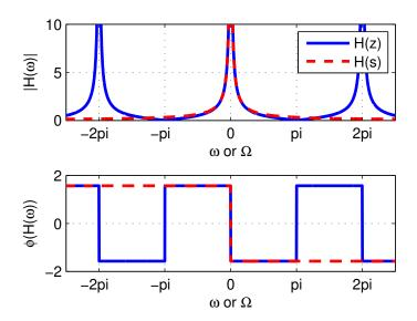
On the interval  $[-\pi, \pi]$ , the responses are nearly identical; outside this interval,  $H(\omega)$  is periodic but  $H(\Omega)$  is not.
