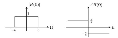
Consider a continuous-time LTI system of which the frequency response is shown above.
