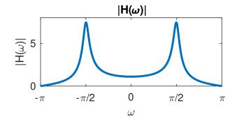
Close to poles, the response peaks. At  $\omega = \pi$ , the response is zero because there is a zero at z = -1. At  $\omega = 0$  (z = 1), the response is not zero, but not very big either. Calculate  $H(e^{j0}) = 2/1.81 = 1.11$ .
