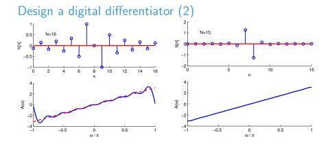
An odd filter order N (type IV) results in a much faster decay of h[n], because of the square in the denominator.
