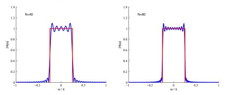
A larger N results in a smaller transition band, but the ripples have equal magnitude! This is the Gibb's effect.
