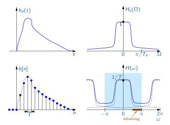
This technique is not suitable for high-pass characteristics because of aliasing.
