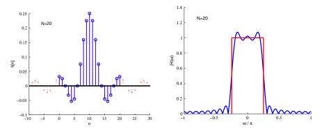
The pass-band and stop-band are OK, but the ripples are too large.
