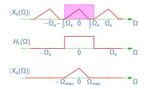
The reconstruction filter eliminates the extra copies; the original signal is recovered.
