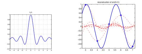
The sinc-functions take care of the interpolation. Note the locations of the zero crossings of the shifted sinc-functions.
