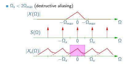
The part of the spectrum beyond  $\pm \frac{1}{2}\Omega_s$  is apparently "folded back".
