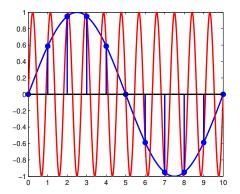
The red signal has  $\Omega_0 > \frac{1}{2}\Omega_s$ , after sampling the signal is identical to that of the blue signal for which  $\Omega_0 < \frac{1}{2}\Omega_s$ .
