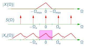
The part of the spectrum beyond  $\pm \frac{1}{2}\Omega_s$  is apparently "folded back".
