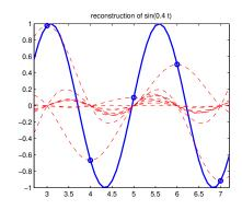
The sinc-functions take care of the interpolation. Note the locations of the zero crossings of the shifted sinc-functions.
