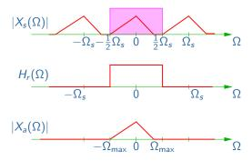
The reconstruction filter eliminates the extra copies; the original signal is recovered.
