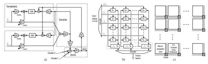
Figure 1: a) Conceptual diagram of the neuromorphic synapse, and a dendrite (input) and an axon soma (output) of a biological neuron, b) Internal blocks of the neuromorphic core with dedicated synapse, c) High-level architecture for learning systems with an array of neuromorphic cores.
