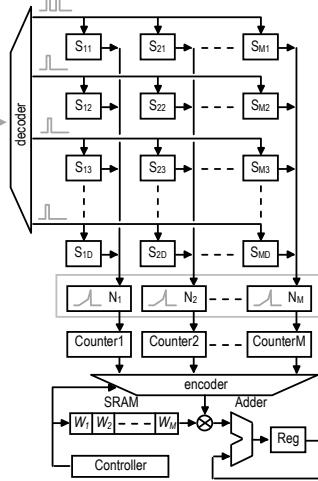
Figure 1: Overview of the neuromorphic core including adaptive, integrate-and-fire neuron-, and synapse circuits, respectively, SRAM, adder, multiplier, register and controller.
