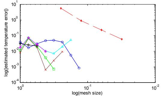
Figure 3: Estimated temperature error versus mesh size for the proposed (several  $G_{(aged)}$  bold lines), and generalized finite element method (red dashed line); neuromorphic processor interconnect example.
