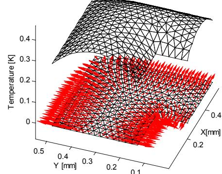
Figure 2: Temperature profile of neuromorphic processor interconnect at the (critical) crossings. Thermal expansion and aging effects are illustrated with arrows.
