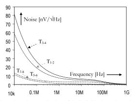
Figure 8: Noise contribution of the individual transistors in the OTA
