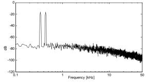
Figure 10: Spectral signature of programmable gain A/D converter-two tone test.
