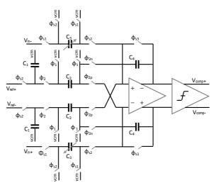
Figure 2: Schematic of programmable gain ADC.
