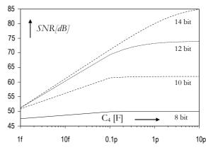
Figure 3: Maximum achievable SNR for different sampling capacitor values and resolutions.
