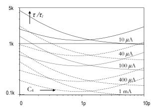
Figure 5: Closed loop normalized time constant versus hold capacitance  $C_H$  for different biasing conditions; case for  $C_4=3C_L$ ,  $C_L=C_p$ . The time constant is normalized to the  $\tau_t$  (=1/f<sub>t,intrinsic</sub>) of the device, which is approximately ( $C_G/g_m$ ).
