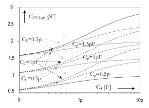
Figure 6: Optimum gate capacitance  $C_{OTA,opt}$  versus hold capacitance  $C_4$  for different loading and parasitic conditions.
