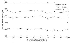
Figure 12: SFDR, SNDR and THD versus sampling frequency with  $f_{in}$ =5 kHz and gain set to one.
