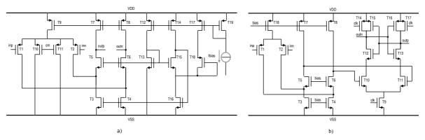
Figure 7: a) OTA schematic, b) Comparator schematic.
