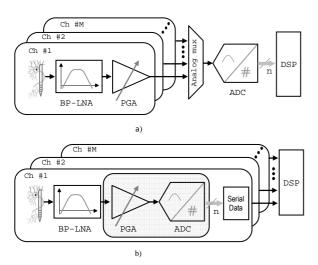
Figure 1: Multichannel neural interfaces: a) Multiplexing an ADC between M channels, b) An ADC per channel with serial interfacing.
