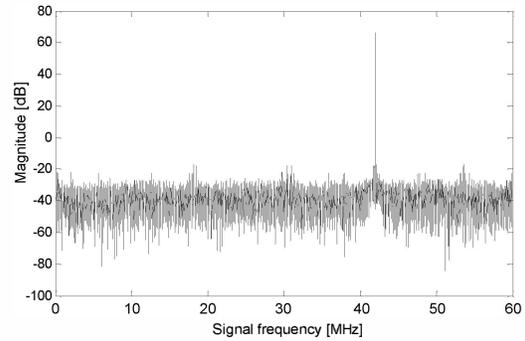
Figure 3: Measured spectrum the time-interleaved S/H at 120MS/s
