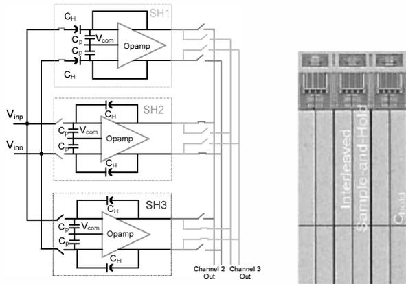
Figure 1: Left) Total S/H circuit consisting of three time interleaved S/H units at the moment when S/H1 is sampling and S/H2 and S/H3 are holding. Right) Chip micrograph.
