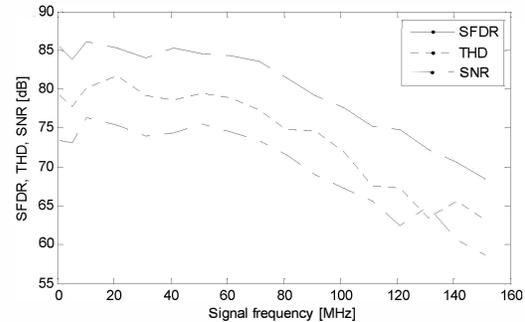
Figure 4: Measurement result of the time-interleaved S/H at 120MS/s
