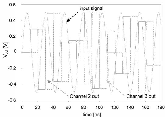
Figure 2: Simulated time domain sample and hold output.
