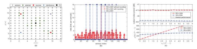
Figure 1. (a) The experimental setup, where the green sensors are selected by the sensor selection method with  $\alpha = 0.6$ , (b) an example for rate distribution with  $\alpha = 0.6$ , (c) noise reduction performance and energy usage in terms of the normalized microphone self-cost with  $\alpha = 0.6$ .
