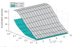
Figure 2. The cardinality of the activated sets of the two approaches in terms of  $\alpha$  and sensor self-cost.
