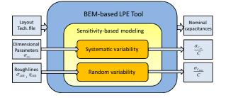
Fig. 6. Diagram of the proposed sensitivity-based method integrated in BEM-based LPE tools for both systematic and random variabilities.
