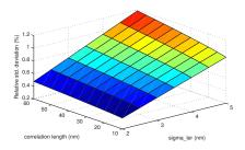
Fig. 3. The mismatch  $(\frac{\sigma_C}{C})$  versus  $\sigma_{LER}$  and  $\eta_{LER}$  for a pair of 200nm long conductors.
