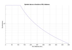
Figure 11. Symbol rate vs ISL distance using UHF link.
