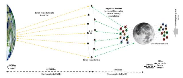
Figure 5. Hybrid fractionated swarm architecture.
