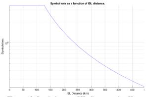
Figure 13. Symbol rate vs ISL distance using Kaband for HDR-ISL (Intra-swarm)
