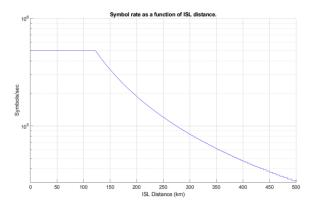
Figure 10. Symbol rate vs ISL distance using S-band for LDR-ISL.
