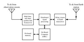
Figure 6. Functional block diagram of communication relay swarm.
