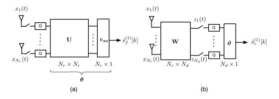
Fig. 2: (a) Full rank Wiener beamformer, (b) reduced rank beamformer interfering users. The desired user estimate can be obtained through digital post-processing  $\hat{s}_r^{(1)}[k] = \vartheta^H \mathbf{z}[k]$ , where  $\vartheta$  can be computed using a training sequence.
