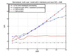
**Fig. 4**: SINR performance improvement due to the APN array have SINR of -6 dB (curve 1) and APN (curve 2) improves the SINR to -1.7 dB (for input SNR: $10 \sim 20$  dB). Curve 3 shows the APN followed by baseband processing in reduced rank, results in approximately the same MMSE as that of full rank processing (curve 4).
