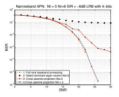
**Fig. 5**: BER performance comparison of the APN major power spending unit in the receiver, these results provide significant insight into translating the theoretical performance of MIMO systems in practice.
