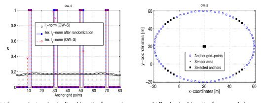
(a)  $\ell_1$ -norm (not randomized) and *iterative*  $\ell_1$ -norm (randomized). **Fig. 2:** Anchor placement for OW-S, for  $P_e = 0.95$ ,  $e_s = 10$ J, and  $R_e = 5$ cm.
