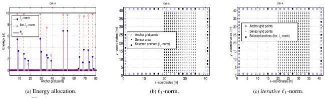
Fig. 1: Joint anchor placement and energy optimization for OW-A, for  $P_e = 0.95$ ,  $e_b = 10$ J, and  $R_e = 4$ cm.
