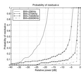
Figure 2: Probability distribution of relative residual power. BW = 25 kHz, 270 kHz, 1 MHz, 5 MHz. FM chirp.
