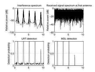
Figure 3: (a) Interference spectrum. (b) Noisy signal spectrum. (c) Detection probability vs. frequency for LRT, and (d) for MDL.
