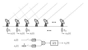
Figure 1: Schematic of the Westerbork radio telescope
