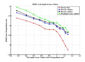
Fig. 2. The relative mean square errors in the computed short-circuit capacitance matrices.
