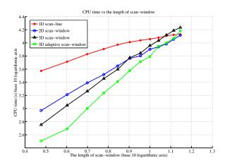
Fig. 3. The CPU time needed to computed the short-circuit capacitance matrices Vs the scan-window size.
