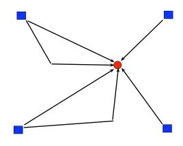
Fig. 1. Four base stations with multiple ranges towards the mobile station
