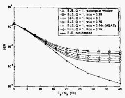
Fig. 4. BER of MMSE-BLE with different SOE windows  $(Q=1, f_D/\Delta_f=0.15).$
