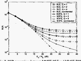
Fig. 2. BER comparison between MMSE-BLE and MMSE-BDFE  $(f_D/\Delta_f \approx 0.15)$ .
