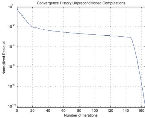
Figure 3: Convergence history of unpreconditioned GMRES for an inhomogeneous slab with  $d = 4\lambda_0$  and dip = 8.
