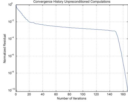
Figure 1: Convergence history of unpreconditioned GMRES for a homogeneous slab with  $d = 4\lambda_0$  and a contrast  $\chi = 128$  (dip = 0).
