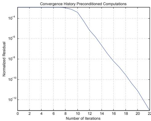
Figure 4: Convergence history of preconditioned GMRES for an inhomogeneous slab with  $d = 4\lambda_0$  and dip = 8
