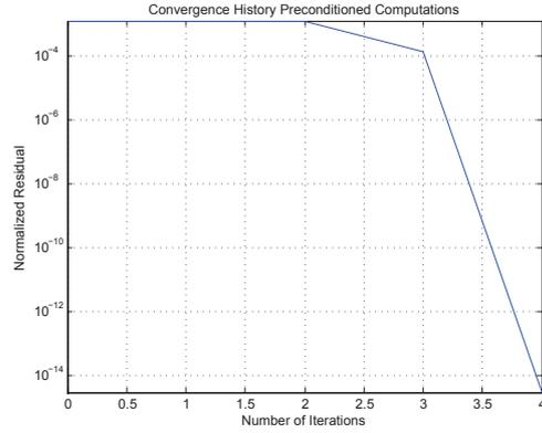
Figure 2: Convergence history of preconditioned GMRES for a homogeneous slab with  $d = 4\lambda_0$  and a contrast  $\chi = 128$  (dip = 0).
