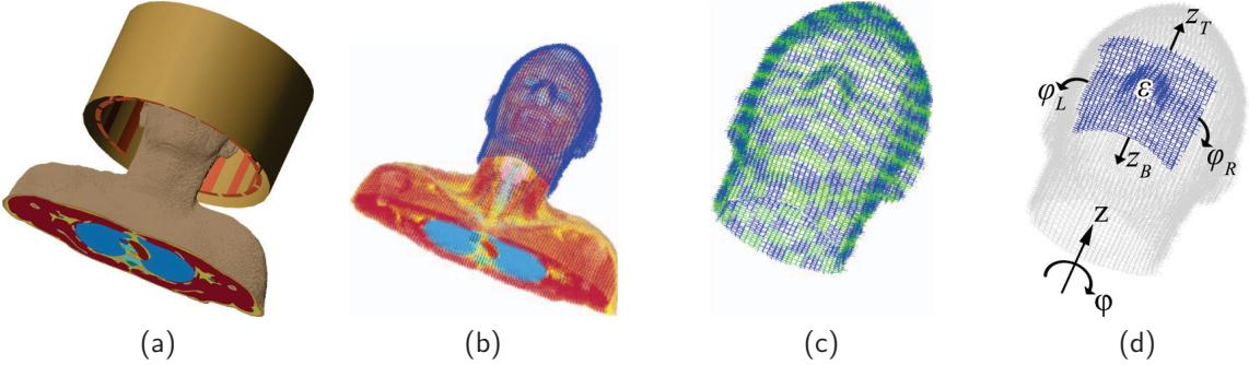
Figure 2: Head and shoulders of the male body model Duke, head coil, and shield used for enhanced imaging of the cerebellum (a). The pad design domain defined all around the head model (b). Pad design domain subdivided into subdomains (c). Illustration of the pad design parameters (d).
