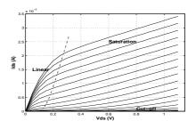
Fig. 2. The nonlinear properties of minimum-sized NMOS device
