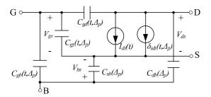
Fig. 1. The proposed SXmodel for gate modeling
