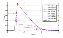
Fig. 8. Waveform evaluation of the NAND4\_X1 cell
