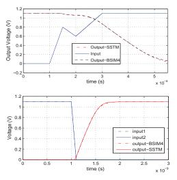
Fig 4 Top: irregular input; Bottom: simultaneous multi-input switching for a 2-input NAND gate
