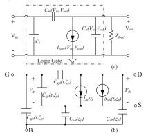
Fig 2 a) Current-source model; b) Proposed SSTM
