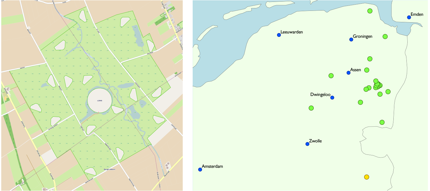
Fig. 2. Geographic distribution of LOFAR stations within the Netherlands. Left: this panel shows the distribution for the majority of the stations within the LOFAR core. The central, circular area contains the six Superterp stations described in the text. The white, polygonal areas mark the location of LOFAR core stations. In addition to the Superterp stations, 16 of the remaining 18 core stations are shown. Right: this panel shows the distribution of remote stations within the Netherlands located at distances of up to 90 km from the center of the array. Stations shown in green are complete and operational while yellow depicts stations that are under construction as of March 2013 (see Sect. 14.1).
