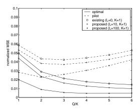
Figure 1: Effect of increasing the smoothness of the window when critical sampling is employed.
